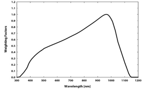
Spectral response estimate of Apogee silicon-cell pyranometers.
